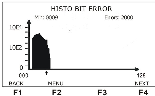
There is a small cursor immediately below the graphic which points to a column. In the upper part of the display, just below the title, there is the minute or hour that corresponds to the column pointed to by the cursor and the number of errors or alarms that happened per minute. To move the cursor through the graph, use the → or ← keys to move the cursor a column at a time, or the ↑ or ↓ keys to move the cursor 16 positions at a time.
