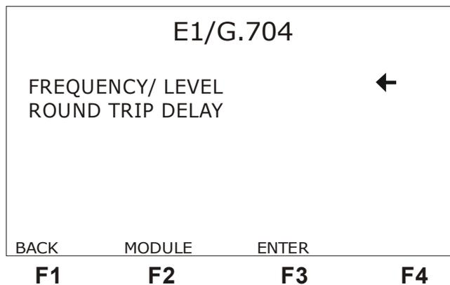
To alternate between these two menu screens, use <F4> (MORE) or <F1> (BACK). Press <F2> (MODULE) to go back to the Module screen.
