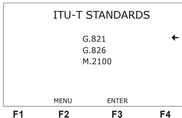
The user can choose the analysis to be displayed, placing the cursor appropriately and pressing <F3> (ENTER).
