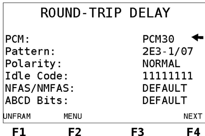
The setup for structured mode has three screens. To navigate among the screens use <F4> (NEXT) and <F1> (BACK) keys. A description of the setup parameters for the Round-Trip Delay mode follows.
