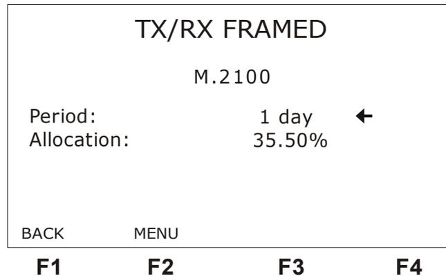
The TSW200E1 calculates parameters following ITU-T Rec. M.2100. The user must preset these parameters. This configuration establishes the test time for M.2100. The TSW200E1 tests up to 8 periods. After that, it starts to write over the old tests. That means that at each 8 periods the TSW200E1 starts a new cycle.
