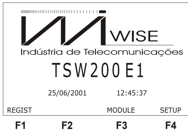
It is then possible to check the equipment register pressing <F1> (REGIST). This screen displays the hardware and software versions and the equipment serial number.
