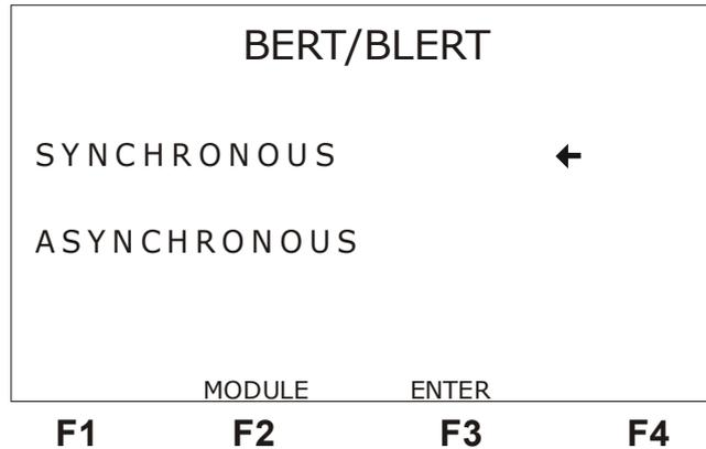
To choose between one of the two modes move the cursor, with the ↑ and ↓ keys, to the corresponding desired mode and press <F3> (ENTER). The first screen for the chosen module setup will be displayed.
