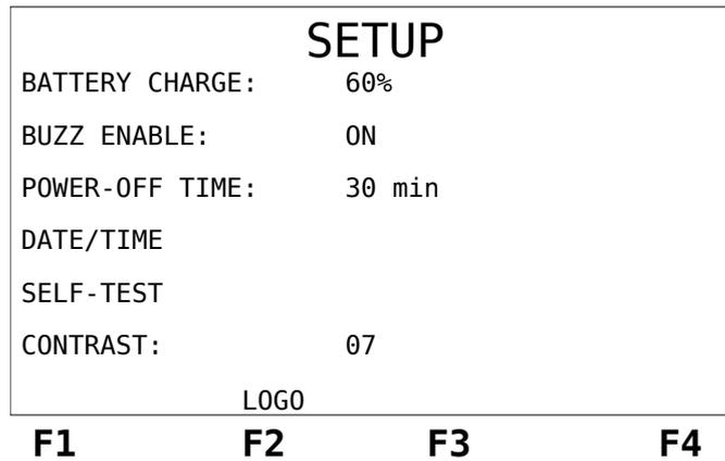
It is possible to turn the keyboard, alarms and error buzzer on or off. To do that, move the cursor to the Buzz Enable line and use the ← and → keys to toggle between ON or OFF. When the buzzer is on, a beep sounds when any key is pressed.
