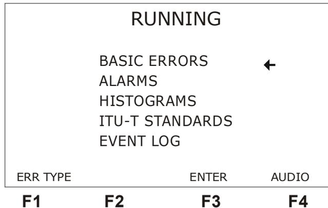
When the CLEAR key is pressed, the test time, all counters and histograms are cleared and the test is restarted. If the TSW200E1 was in sync, it remains in sync.
