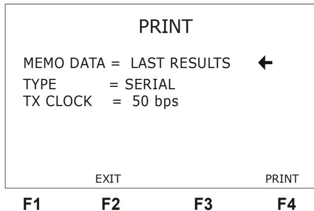
Use the ↑ or ↓ keys to place the cursor at the appropriate line and use the ← or → keys to set up the parameter as desired. Place the cursor at the MEMO DATA line and select the data source (last test result, LAST, or memories 1 to 10, MEMO1 to MEMO10). After that, select the print TYPE and the data transmission speed in TX CLK. After this, press PRINT or <F4> and the results will be printed. To get out of this screen, press <F1> (BACK).
