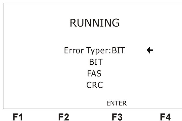
In this screen it is possible to select the type of error inserted when the <ERROR> key is pressed. To select the kind of error, move the cursor to the appropriate line and then press <F3> (ENTER).
