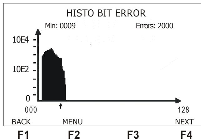
There is a small cursor just below the graph that points to a column. In the upper part of the display, just below the title, there is the minute or hour that corresponds to the column where the cursor is. There is also the number of errors or alarms (according to the plotted graph) that occurred on that particular minute. To move the cursor through the graph, a column at a time, use the → and
