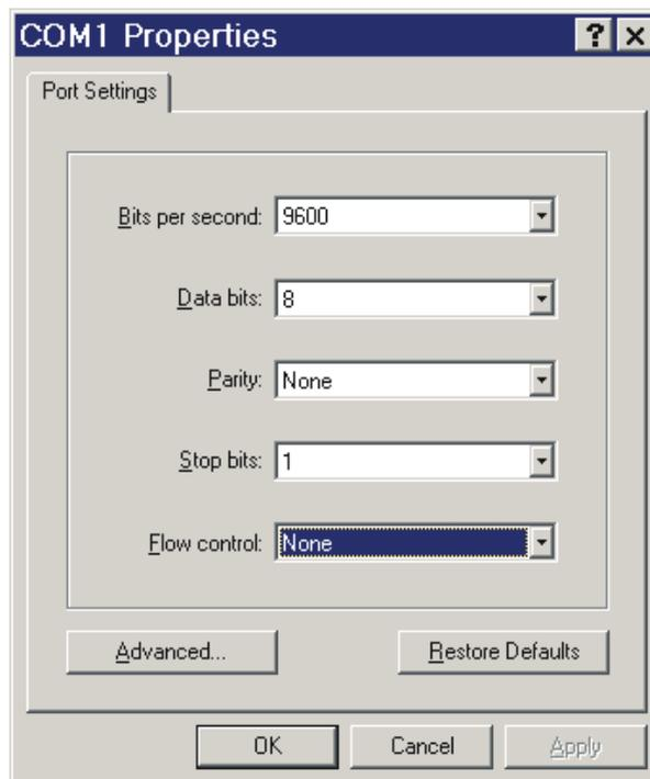
From this moment on, the computer will receive data by the selected serial port. At the TSW200E1, press the PRINT or <F4> key and the data will be sent to the computer. The ASCII-only text appears in the screen.
