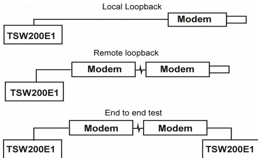
After making connections and after setting up the configuration parameters, press the START/STOP key to start the test. If the CTS circuit is active, the Test Set will continuously transmit the selected pattern. The RUN indicator LED will remain on while the test is running. If the test is continuous, press START/STOP to stop the test.
