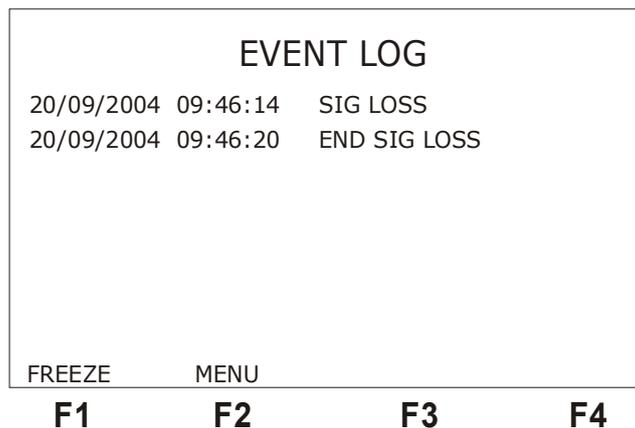
To go back to the menu screen, press <F2> (MENU). By pressing <F1>(FREEZE) the screen is not updated anymore. Over the <F3> key the number of the last line shown on screen is displayed. Over the <F4> key the total log lines is displayed. With the ← and → keys it is possible to go to the start or to the end, respectively, of the log. The ↑ and ↓ keys display the previous or the next line. To update the screen again, press <F1> UPDATE.
