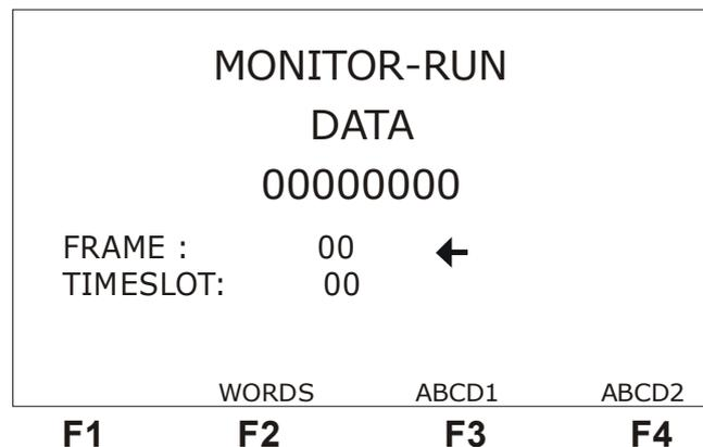
In this screen it is possible to monitor the selected timeslot and frame data. During the test it is possible to select another timeslot and frame to be monitored. To do this, move the cursor appropriately with the ↑ and ↓ keys. Use the ← or → keys to change the number of timeslot or frame.
