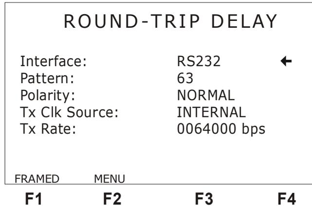
To toggle to the structured circuits setup screen, press <F1> (FRAMED). The following screen will be shown:
