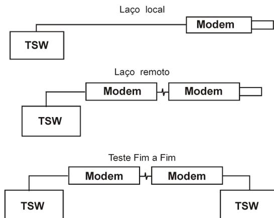
Figura 4 .13: Bit Error Rate Test/ Block Error Rate Test
