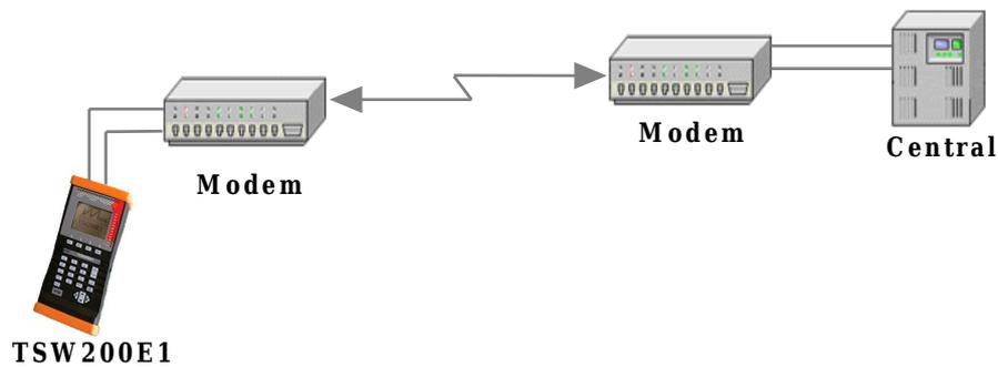
TSW200E1 connected as MONITOR
