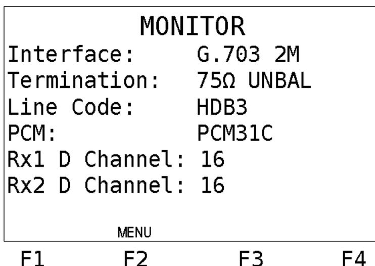
To use the Monitor mode, the user must connect the two transmission signals to the two receive terminals (RX1 and RX2), which are available at the TSW200E1. It is recommended to select the High-Z impedance mode.
