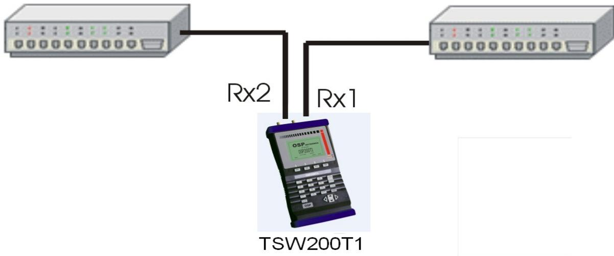
Figure 2: TSW200E1 connected as terminal.
