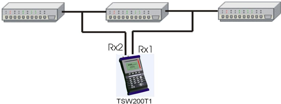
Figure 3: TSW200E1 connected as monitor (high impedance - Hi-Z).
