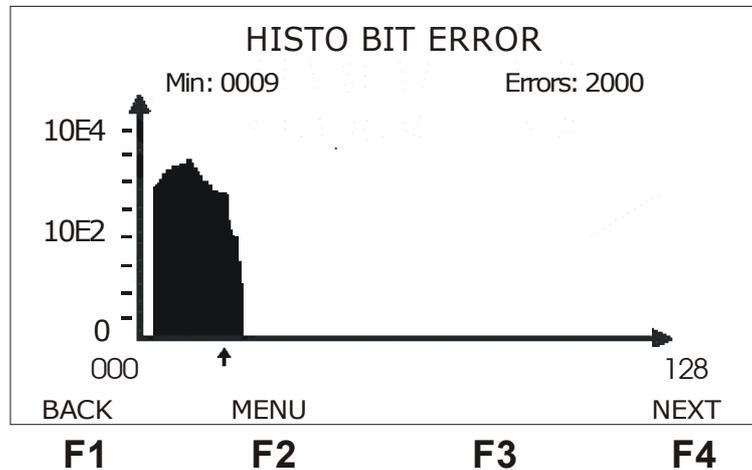
There is a small cursor below the graphic that points to the column. In the upper part of the display, right below the title, there is the minute or hour corresponding to the column pointed to by the cursor and the number of errors or alarms that occurred in that minute (according to the plotted graphic). To scroll the cursor over the graphic, use the ← and → keys to move the cursor on a column basis or the ↑ and ↓ keys to move the cursor 16 positions at a time.
