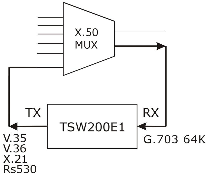
The test consists in sending a data pattern and checking if this same pattern is received in the X.50 frame structure. The test pattern is sent to the multiplexer via the interface that can be user-chosen as V.35/V.11, V.36/V.11, X.21/V.11 or RS530. The reception of the X.50 data stream is always through the G.703 64kbps (Codirectional) interface.
