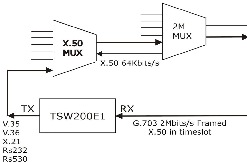
The test consists in sending a data pattern to the X.50 multiplexer and checking this same data pattern within the X.50 structure inserted in a PCM slot. In that way, the data pattern is sent via the interface chosen at the configuration screen and the reception is done by the G.703 2M interface.
