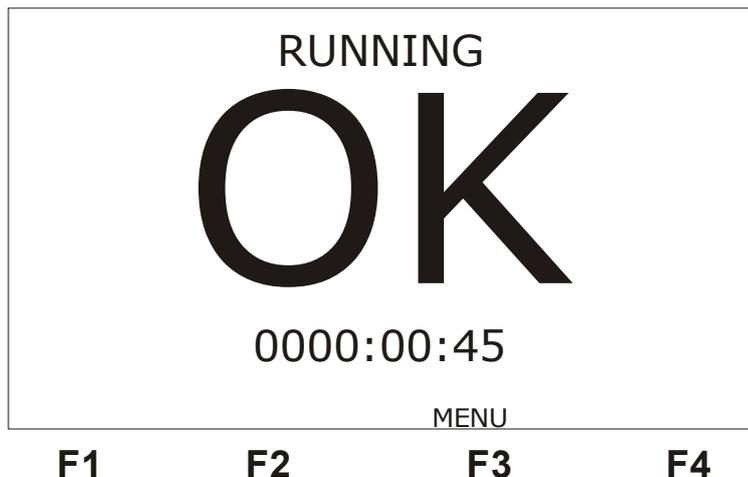
When detecting an error or alarm, the test set automatically changes the screens, displaying the error or alarm counter. From the moment the error or alarm is detected, the OK screen is not accessible anymore.
