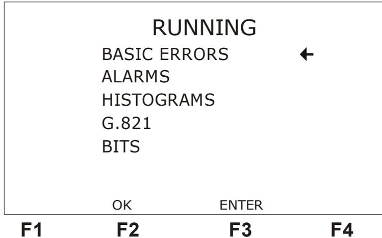
From this screen, it is possible to access the error, alarm, histograms, G821 analysis or bit screens. To do this, move the cursor to the appropriate line and press <F3> (ENTER).
