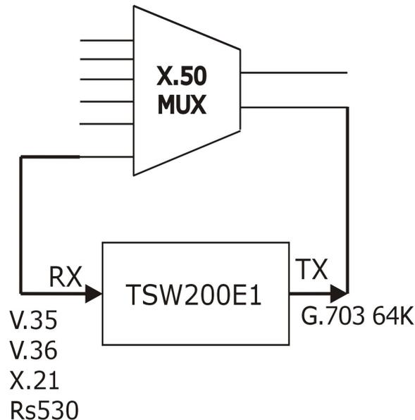
The test consists in sending a data pattern in the X.50 frame structure and checking if that same pattern is received at the chosen interface. The X.50 data stream transmission carrying the test pattern is done via the 64k G.703 interface. The test pattern is received from the demultiplexer, via the V.35/V.11, V.36/V.11, X.21/V.11 or RS530 interfaces.
