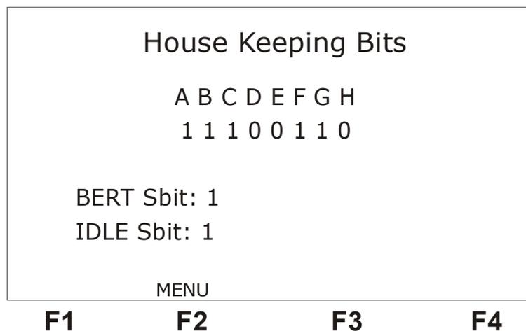
This screen allows visualisation of the maintenance bits (A, B, C, D, AND, F, G and H), which are being received and the BERT/IDLE Sbits status. If division 3 is chosen, only the A and BERT/IDLE Sbits bits are displayed. Press <F3>(MENU) to go back to the OK screen or to the MENU screen.
