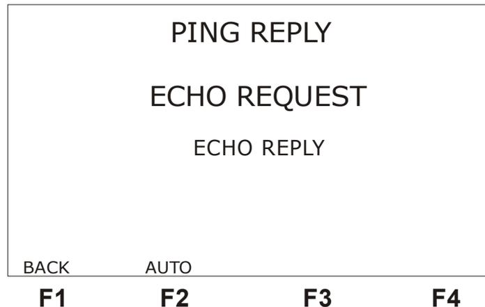
When the test set receives an ECHO REQUEST, this expression is displayed in large letters on the screen. When it responds, the expression ECHO REPLY is displayed in large letters on the screen. If there is only ECHO REQUEST, it is likely that the received IP address is different from the configured Source IP Address. In this case, the TSW200E1 does not generate ECHO REPLY, but it signals that it received an ECHO REQUEST.
