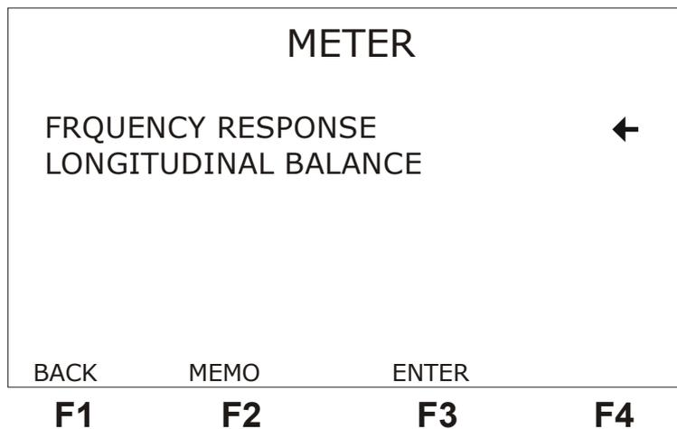
From these screens, it is possible to choose one of the modes for configuring and operating the equipment. To toggle between the screens, use the F4 (MORE) and F1 (BACK) keys.
