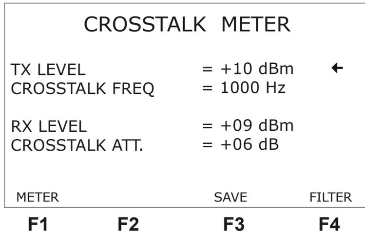
To edit the level and the frequency of the signal to be sent, place the cursor pointing to the value to be changed, use the ← and → keys and press DATA. Within the editing mode, key in the desired value and press F4 (ENTER). The level varies from -50 to +10 dBm and the frequency from 100 to 8000 Hz.
