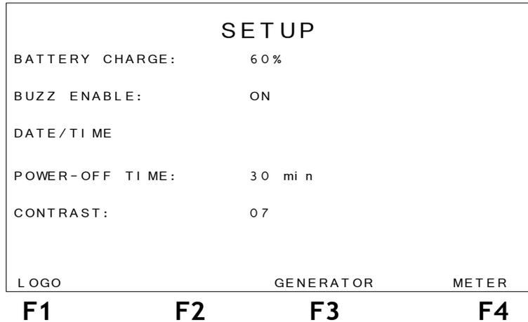
In this screen it is possible to turn on or off the beep by changing the BUZZ ENABLE parameter to ON or OFF respectively. The user can also select the time that the equipment waits to turn itself off in the POWER-OFF TIME parameter as 05, 10, 20 or 30 minutes. Another functionality of the SETUP screen is to alter the display contrast. The equipment date can be edited and the battery charge percentage is also informed.
