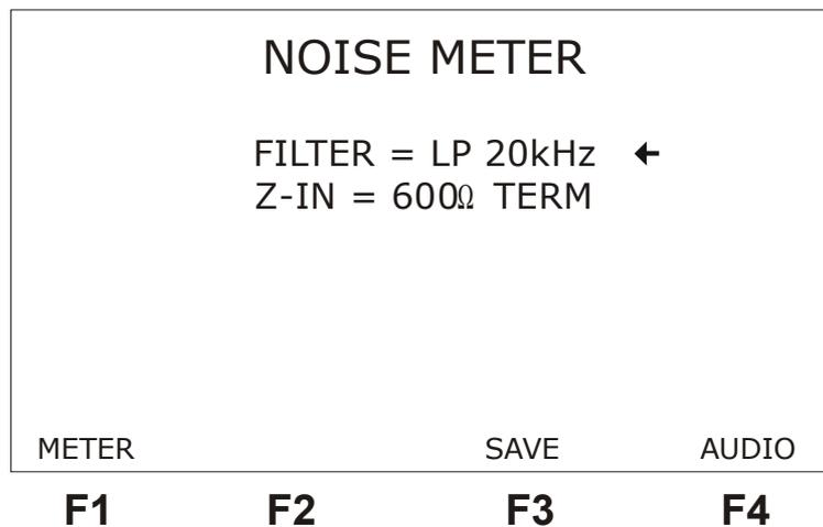
This screen presents two configuration parameters and the results of measuring the noise in dBm. The user can choose the input impedance (Z-IN) and the type of filter to be used, placing the cursor by means of the ↑ and ↓ keys on the appropriate line. To choose the impedance, see section 3.3. To select the desired filter, use the ← and → keys. The TSW300TIM allows using the following filters:
