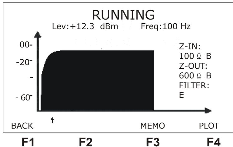
The F4 (PLOT) key allows the test to be run again. The ← and → keys move the cursor to check, in the upper part of the screen, the frequency and level values for each of the graph positions. With the ↑ and ↓ keys, the cursor is moved in 15-step positions.
