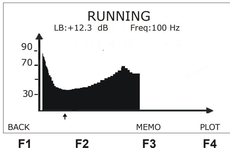
By pressing the F1 (STOP) key, the frequency sweep is interrupted. It can be restarted by pressing the F4 (PLOT) key. When the test is stopped, the user can navigate over the graph, using the cursor. Press the ← and → keys and check on the upper part of the screen the level and frequency values for each of the graph positions. With the ↑ and ↓ keys, the cursor moves 15 steps at a time.
