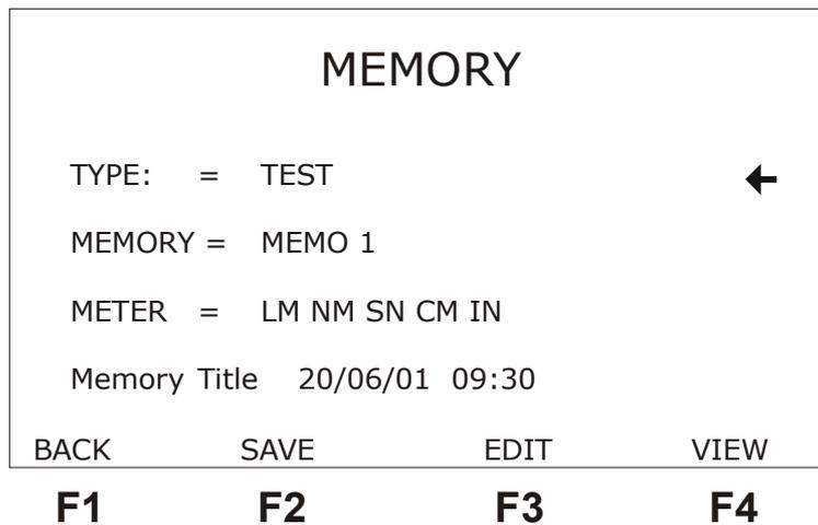
The TSW300TIM memory has 9 (nine) positions to store the graphs obtained in the longitudinal balance and frequency response and 9 (nine) other positions to store the information coming from the other meter tests. For the graphs, the last performed test is stored in position 0 (Last). For the other tests, it is necessary to save the results from each one independently, by pressing the F3 key at the screen for each mode.
