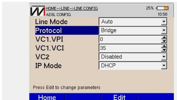
Figure 5.11: Bridge mode configuration
