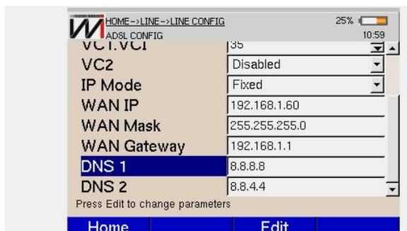
Figure 5.12: Fixed IP configuration
