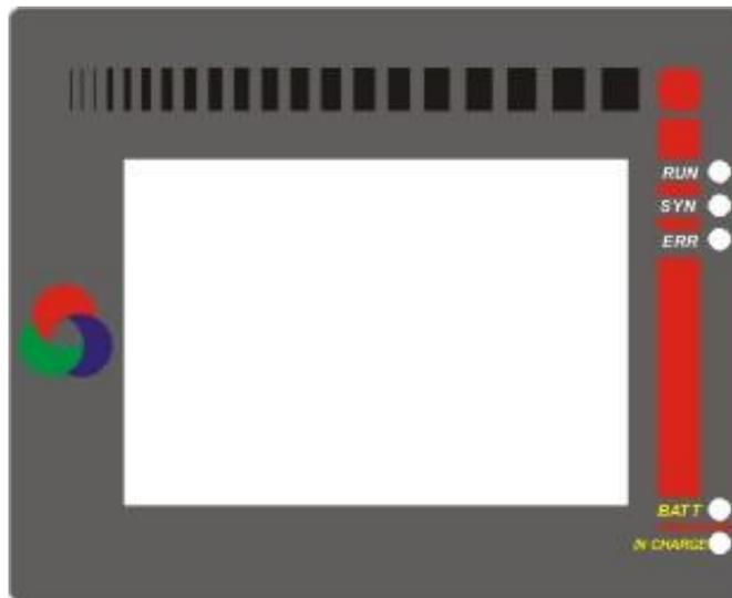
Figure 2.2: TSW800TP LEDs
