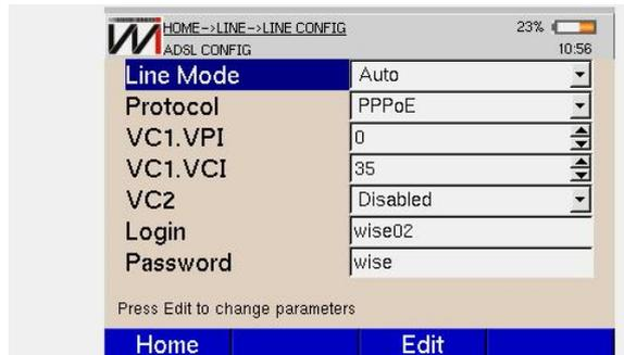
Figure 5.8: xDSL Line Configuration
